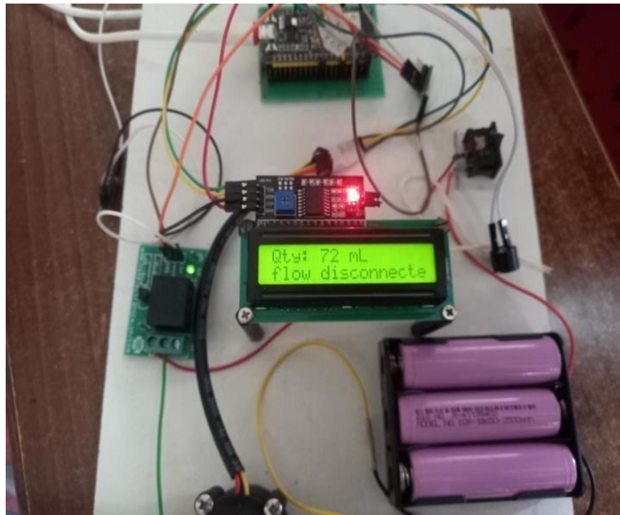
Fig 4.2: LCD display after theft identification Displays the readings of the limit reached on exceeding the limit set
