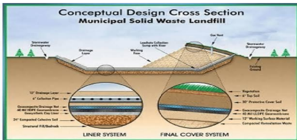
Figure 2.6. Cross section Engineered landfill
