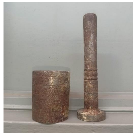
Fig3.4. Mold for making briquette
