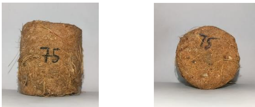
Fig 3.7. 75% areca husk and 25% saw dust briquette
