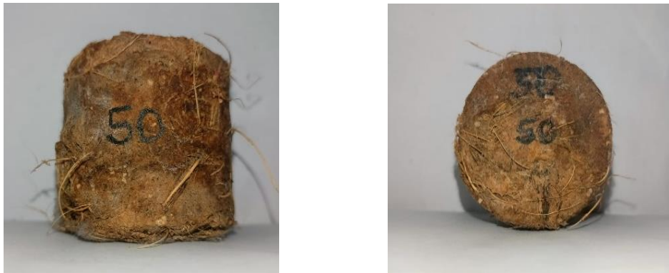
Fig 3.8. 50% areca husk and 50% saw dust briquette
