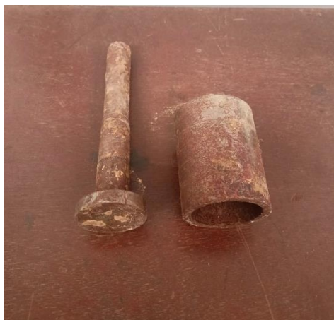
Fig3.4. Mold for making briquette
