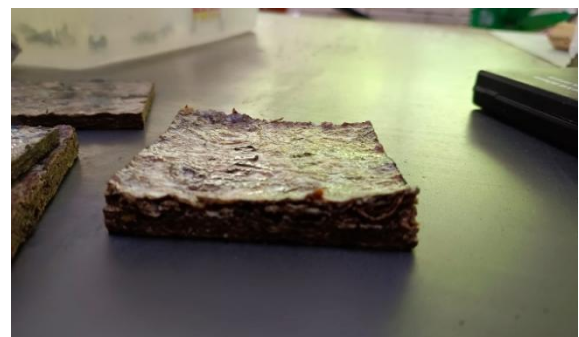
Fig. Water Absorption test Specimen .
