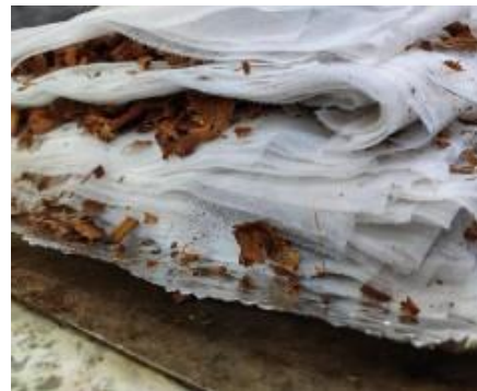
LAYERS OF GNS AND POLYPROPELENE
