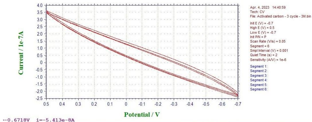
Figure 21: CV curve of Activated Carbon
