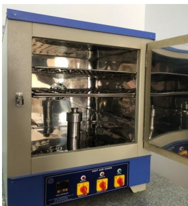
Figure 10: Autoclave reactor inside hot air oven
