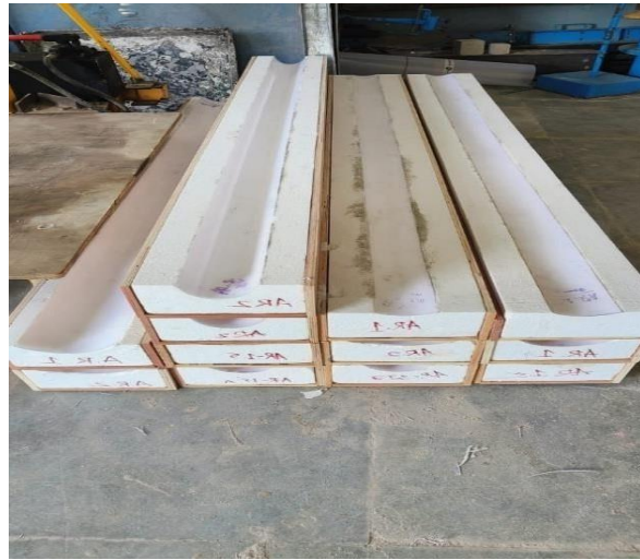
Figure (05) Thermocol supported plywood
