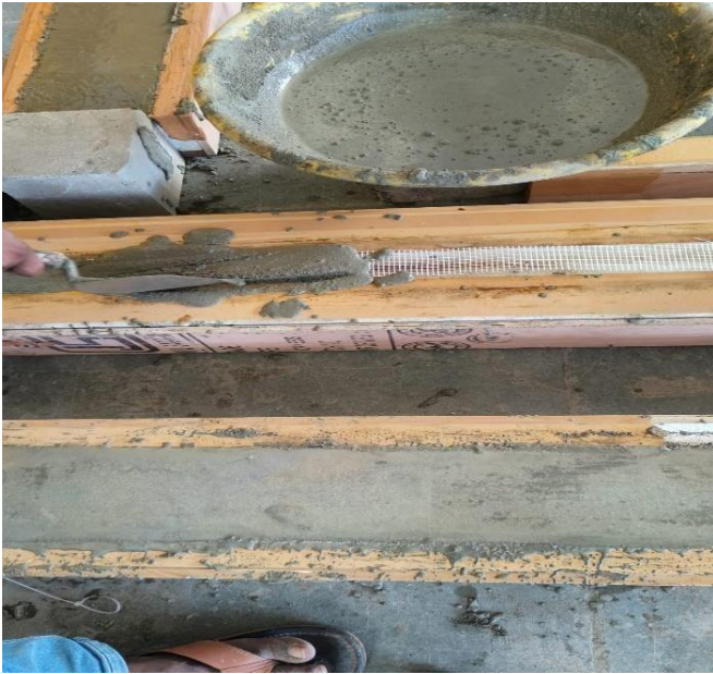
Figure (11) Casting of Specimen
