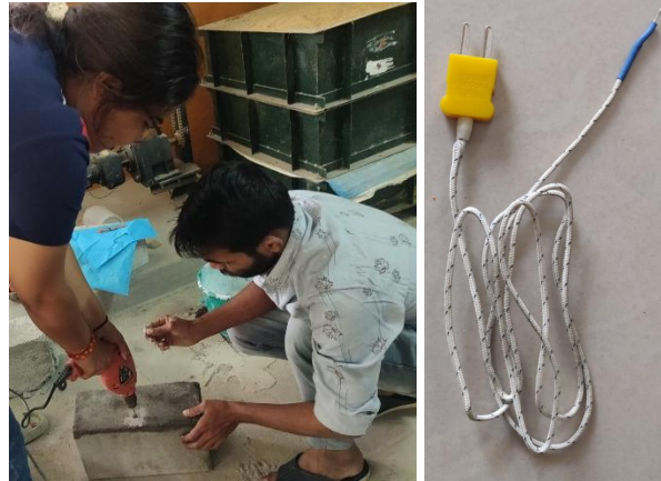
Figure 2.3 - Insertion of Thermocouples in the block
