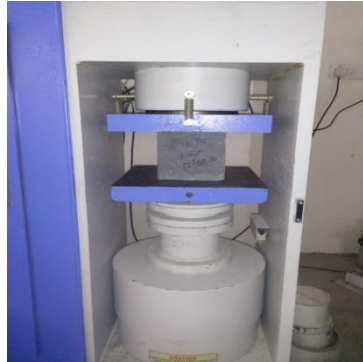
Figure 2.2 - Testing for Compressive Strength in CTM
