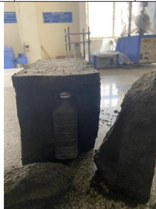
Figure 3.1 - Test specimen after failure
