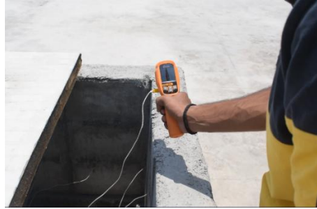
Figure 2.5 - Recording the temperature of thermocouple
