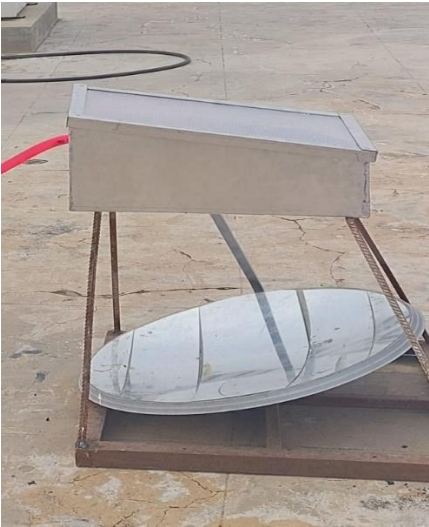
Fig. 7.7 Solar still with parabolic reflector
