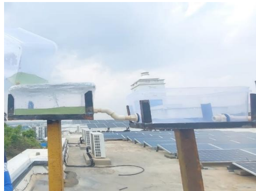
Fig 7.3 Influent tank with bar screens
