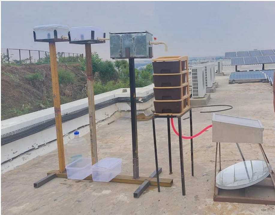
Fig. 7.8 Water Purification Unit
