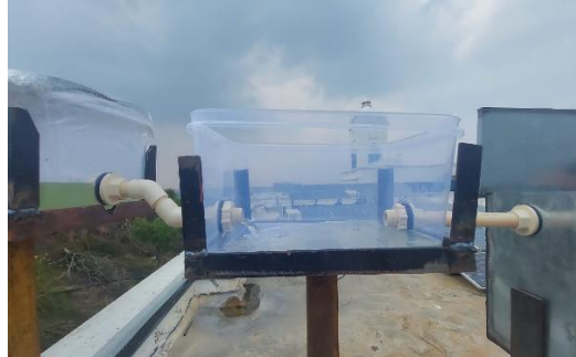
Fig. 7.4 Oil and Grease removal tank
