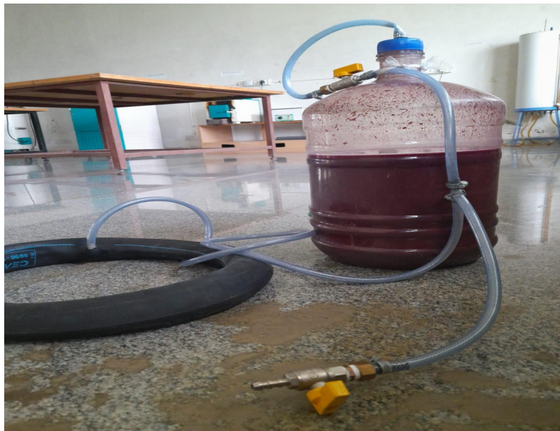
Fig 7.5 Insert the slurry into the digester.
