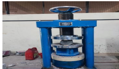
Figure shows the compressive Strength test and Split tensile test.
