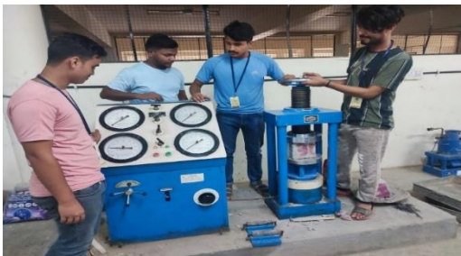
Figure shows the compressive Strength test and Split tensile test.
