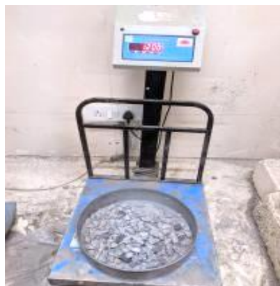
Fig.1 Weighing the proportioned aggregates for DBM
