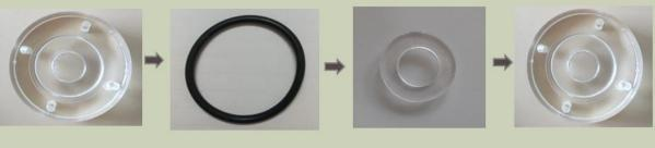
Flange with grooves - 5cm dia , 5mm thickness
