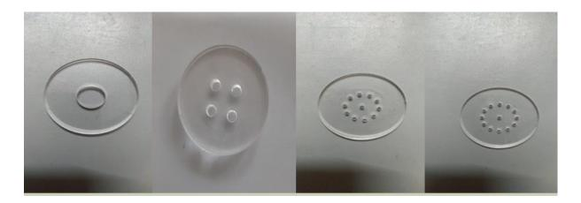
The Conditioning Orifice Plates have four holes that are placed in a circular pattern, leaving a metal section of the plate in the centre of the pipe. This causes the flow to condition itself as it is forced through the holes, thereby removing the requirement for a flow conditioner. Because of this phenomenon, *conditioning orifice plates* provide superior performance in short straight pipe run and tight fit applications.
