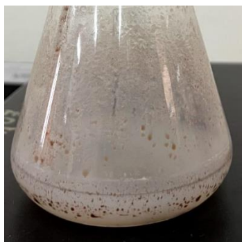
Figure 1: Control sample without fungal spores. It can be observed that the oil has been sticking to the flask surface.
