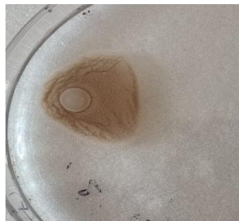
Figure 4: Oil spreading test; Appearance of clear zone on the surface of water.
