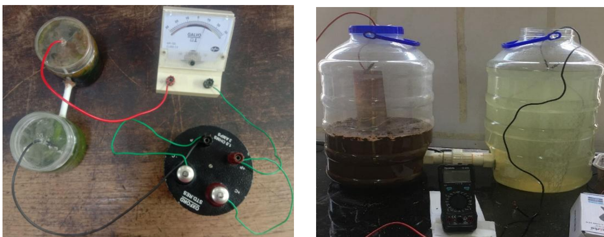
Fig. 2. MFC setups used in the laboratory: (a) MFC with 0.5 kg of food waste, (b) MFC with 5 kg of food waste
