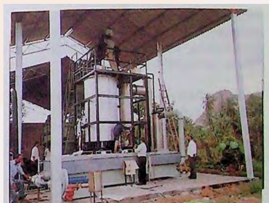
500 kW Biomass gasifier power generation system at M/s Senapathi Whitley Limited, Ramanagaram.
