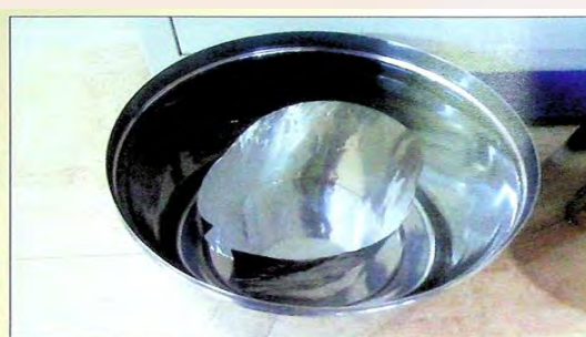
Silver sheet inserted in water sample for testing
