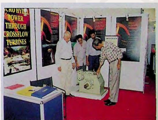
Fig. 1: 50kW crossflow turbine for the microhydel plant at TIRBIN (Arunachal Pradesh)
