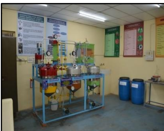
Lab scale transesterification unit Pilot Scale transesterification Unit Separation of organic layer and Glycerol layer
