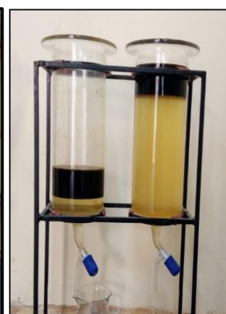
Lab scale transesterification unit Pilot Scale transesterification Unit Separation of organic layer and Glycerol layer
